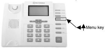
Menu items are selected by using up and down arrow keys  $\blacktriangle \lor$  located below the LCD screen.
