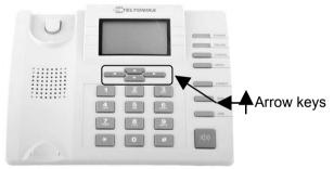
To enter selected menu function press left arrow key  $\triangleleft$  (LCD displays *OK*), to exit press right arrow key  $\blacktriangleright$  (LCD displays *Exit*).
