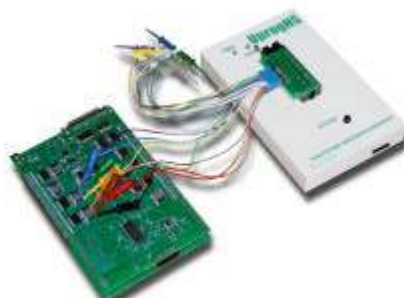
UprogHS 48 USB – logic analyser feature
