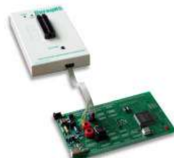
UprogHS 48 USB – in-circuit programming feature
