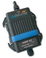
The ARF42 radio modem is a **RS232/WIFI gateway** enabling two-way half duplex wireless data transmission over **200m.** It uses the **2.45GHz** world band according to the WIFI standard.
