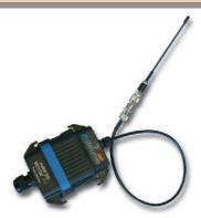
The ARF35 enables two-way half duplex wireless data transmission over a range of 6Km.
